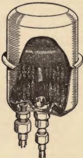
The illustration shows a popular type of oil filter. This is connected to the pressure lubrication system so that the oil is forced up through the centre pipe. Before finding its way to the pipe which returns it to circulation it must pass through the filtering mediums shown.
