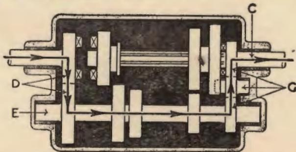
**Reverse Gear.**—Drive follows arrows through constant mesh pinions (d) to lay shaft (e) through reverse pinion set (g), the extra pinion thus reversing the direction of rotation of the second motion shaft (c). In the first two diagrams these reverse pinions have been omitted for the sake of simplicity.
