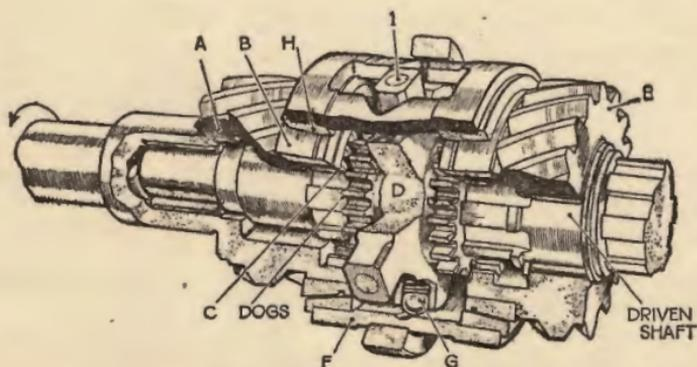
This type of gear enables the speed of two dogs to be synchronised automatically as they are pressed into engagement by the gear lever.
