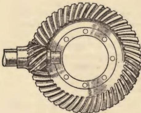
Showing the popular helical or spiral bevel gear. This type of gearing is more silent than the straight bevel once in general use.
