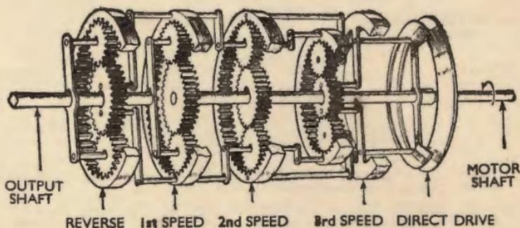
The principle of the WILSON GEAR BOX. When the brake band closes on any one of the drums illustrated and prevents it rotating the Planet wheels must rotate inside the stationary drum and that gear is then in engagement.
