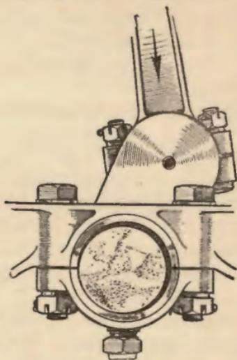
The oil film (shown solid black) which keeps bearing surfaces apart is here shown in an exaggerated form. It can also be seen how the pressure exerted by the explosion, acting through the piston and connecting rod, forces the shaft to one side in the bearing. If the pressure exerted is high enough, and the oil not of good quality, the oil film will rupture and the metallic surfaces will come into contact, causing friction, heat and finally seizure or a “run” bearing.
