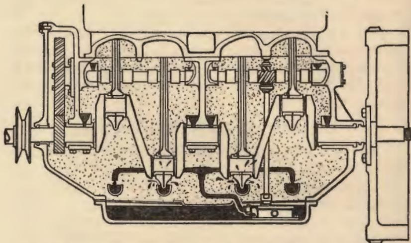
Oil is circulated by pump to troughs beneath the big ends, from whence it is splashed to all parts requiring lubrication, the surplus draining back through a strainer to the sump.
