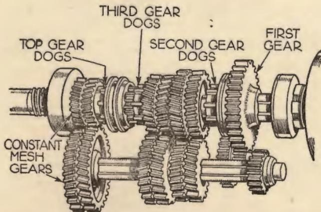
A type of gear box with three sets of constant mesh pinions, or "silent" third and second gears. In top gear, of course, the power is transmitted direct through the main shaft.
