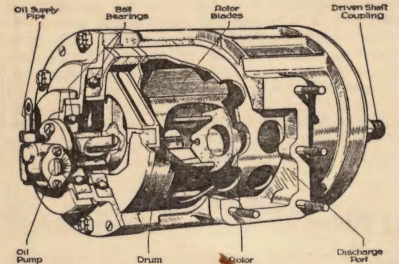
Lubrication connections for superchargers. Sectioned view of the Powerplus Supercharger. (Reproduced by courtesy of Powerplus (1927) Ltd.)
