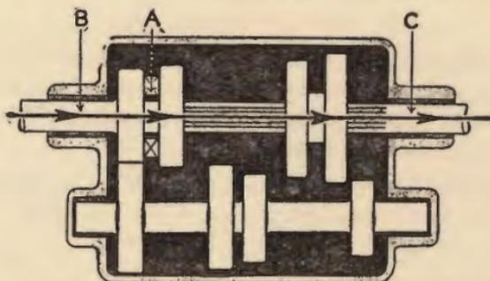
**Fourth or Top Gear.**—Drive follows arrows direct from engine through dog-clutch (a), connecting first (b) and second (c) motion shafts to rear axle.
