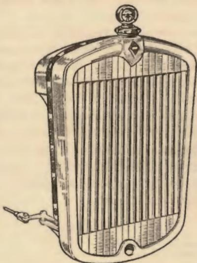
These serve the same purposes as a thermostat valve, but function by shutting off the cooling air instead of restricting water circulation. They may be operated by hand, or automatically by a thermostat.
