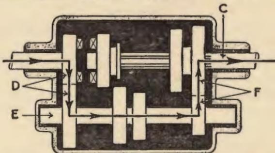
**First or Low Gear.**—Drive follows arrows through constant mesh pinions (d) to layshaft (e), and back through low gear pinions (f) to second motion shaft (c).
