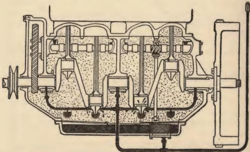
In this system the main crankshaft bearings are pressure fed, the remainder of the engine parts being lubricated as in the simple splash system.
