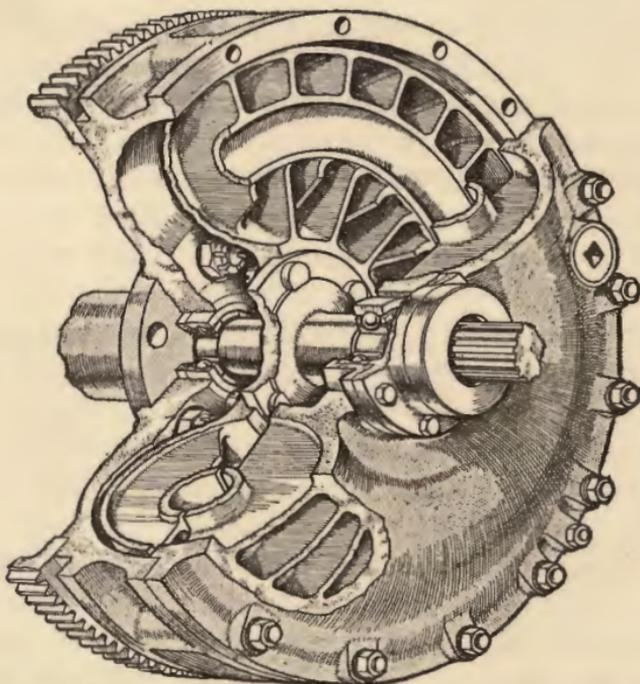
The diagram above illustrates the principle upon which the Hydraulic Clutch of "Fluid Flywheel" operates. Below is a sectional drawing of the actual mechanism showing the simplicity of its construction. (By courtesy of "The Autocar.")
