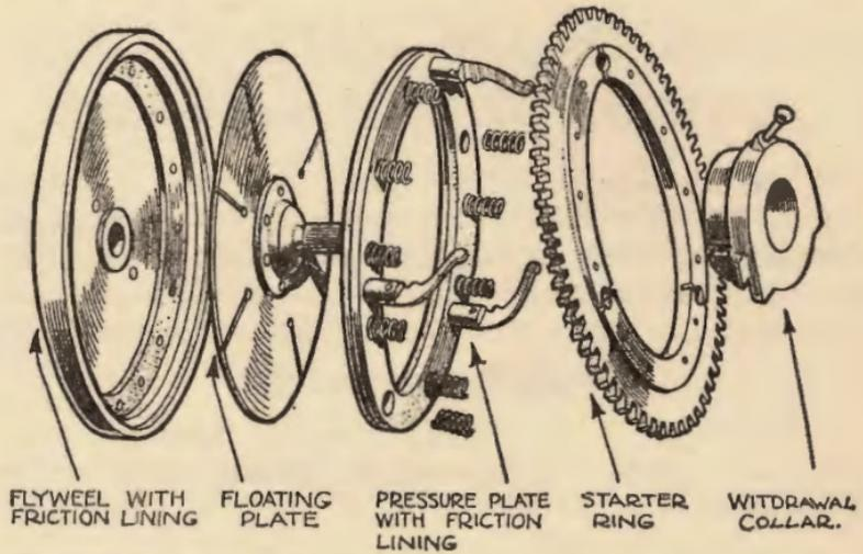
An "exploded" view of the Components of a single plate clutch. (By courtesy of "The Light Car and Cycle-car.")
