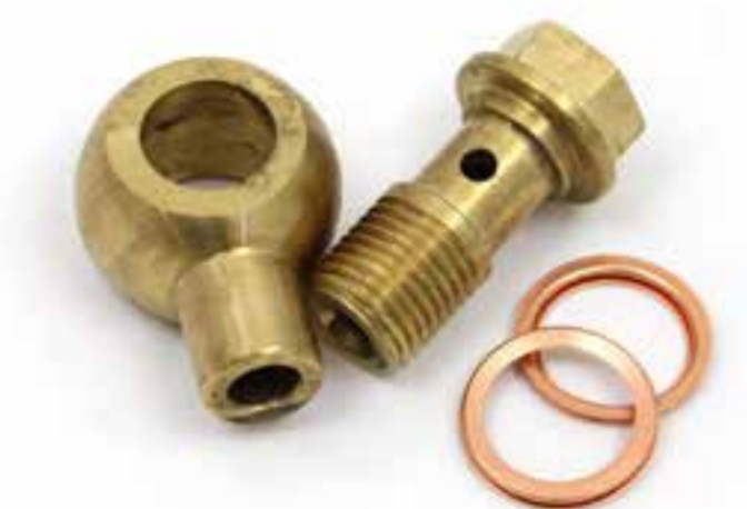
SOLEX carb banjo union, solder 1/4" pipe, M12 x 1.25 thread 368A
