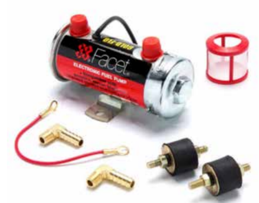
Facet fuel pump 12v Road Neg earth, 18 gallons/hour, 4 - 4.5psi 1337CR
