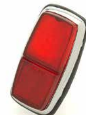
Rear stop and tail lamp, as fitted to AC, Jensen, Hillman. Chrome on brass rim L542
