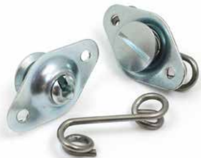
Dzus twist fastener - 16mm reach 38 x 22mm plate, panel fixing, ¼ turn 832B
