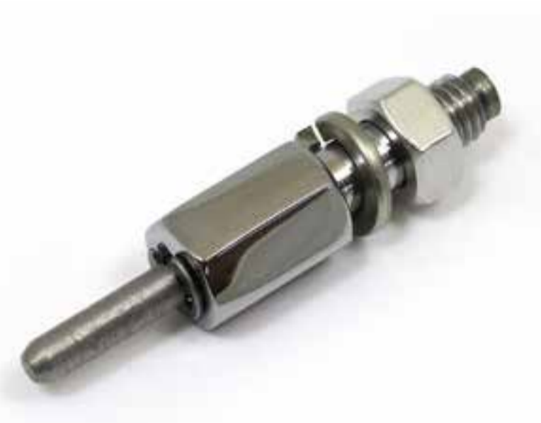
Slave/idle wiper arm pivot, plated brass shaft size 3/16" diameter, 409
