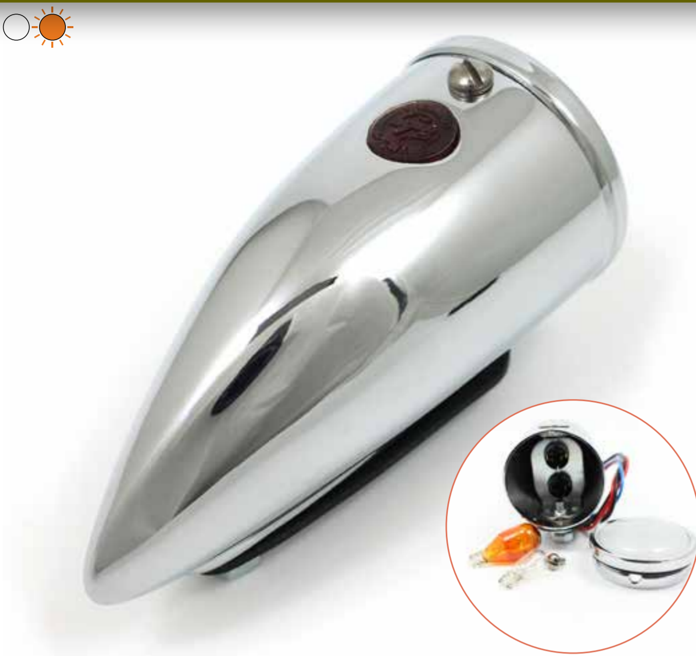
Modified torpedo side/wing lamp with red TOBY 'tell-tale' dot Chrome plated brass body, 2 wedge bulbs - amber & clear 297A-IND
