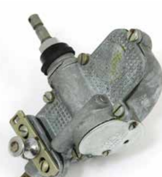
Trico Vacuum wiper motor - NOS Small, windscreen mounted 459
