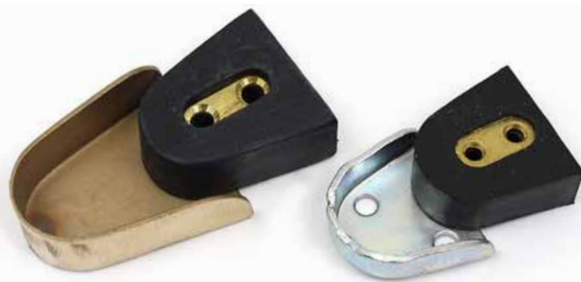
Door buffer wedge - shoe, rubber buffer and screw plate Large cast bronze = 41 x 36 x 14mm deep, small steel = 30 x 30 x 14mm deep 566.08SET, 197
