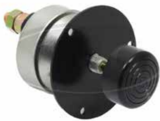
Floor mounted starter switch as Lucas ST18 (076411, also SRB312) CA22
