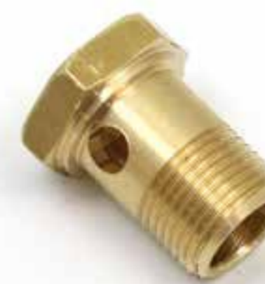
SU carb banjo bolt fits T1, T2 & T4 float chamber lids. 3/8" BSPP thread 368P
