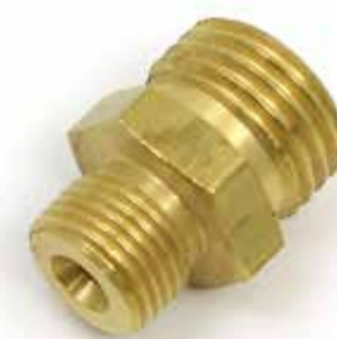
Unequal union, 60° cone seats 1/8" BSP to 1/4" BSP 953
