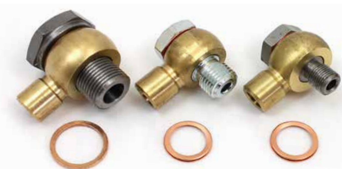
Solder type banjo union with 1/8" BSP with bolt and washers 3/8" BSP for 3/8" pipe, 1/4" BSP for 5/16" pipe, 1/8" BSP for 1/8" pipe 369, 368, 367
