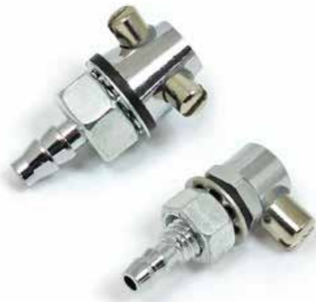
Windscreen washers - small single jet & 13mm diameter twin jet 214S, 214D
