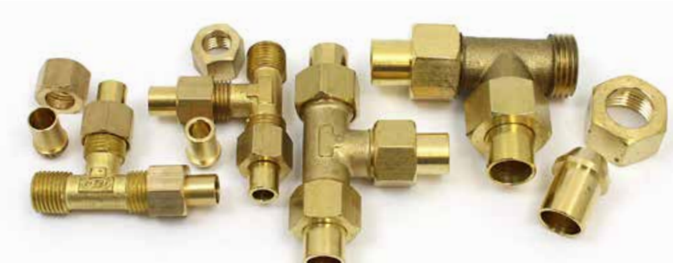
Tee piece kit with solder nipples and nuts for 1/4", 5/16", 3/8", or 1/2" OD copper pipe 345, 346, 347, 347A
