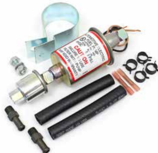
6v Fuel Pump Pos or Neg earth, 5 - 8psi shut off PFP6
